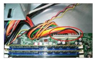
7.2 Disconnect the Audio/FRONT USB/TOP USB/ CARD READER /FRONT cable from the main board
